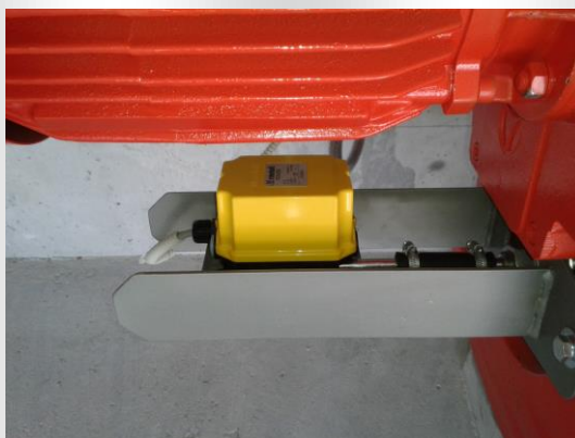
Counter, which allows you to set the upper and lower end position and intermediate position.
