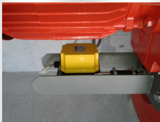
Counter, which allows you to set the upper and lower end position and intermediate position.
